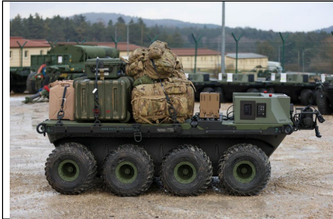
Figure 2. Small Multi-Purpose Squad Equipment Transport INC I , U.S. Army photo by SGT Chandler Coats, “10th Mountain Division implements new drone tech during Combined Resolve 25-1,” January 15, 2025, DVIDS, VIRIN: 250115-A-GR811-3137 (public domain).
