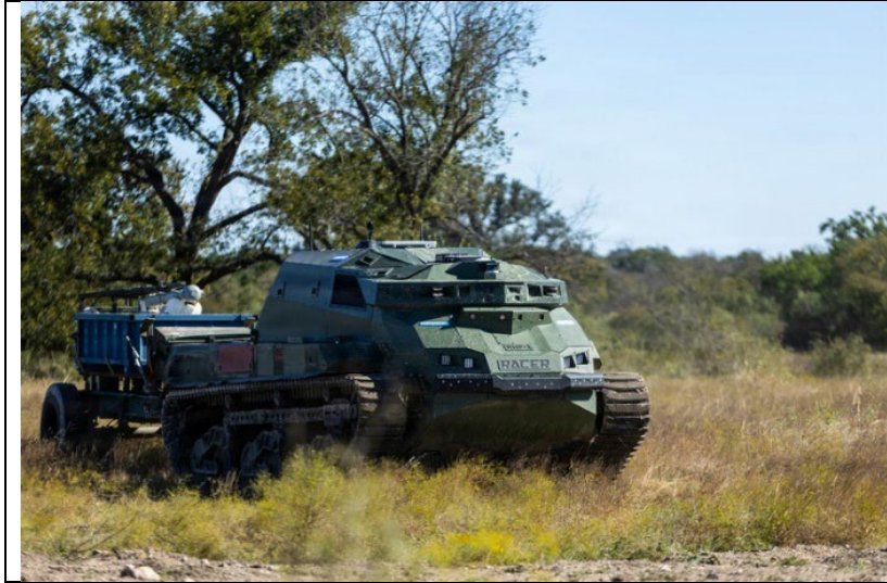
Figure 10. RACER vehicle tows an M58 Mine Clearing Line Charge (MICLIC) during testing in Texas, October 29, 2025. U.S. DARPA photo by Thomas Sakell, DVIDS, VIRIN: 251029-O-GT123-6789 (public domain).
